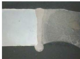
**Fig. 9 (b):** Cross section no undercut with root sagging
