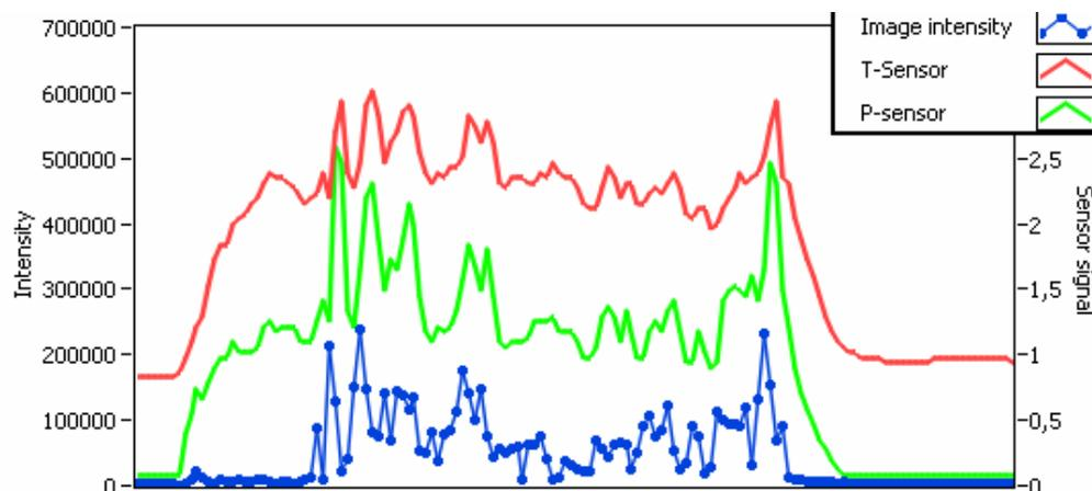
**Fig.11** Calculated image intensity from video and P-sensor/T-sensor
