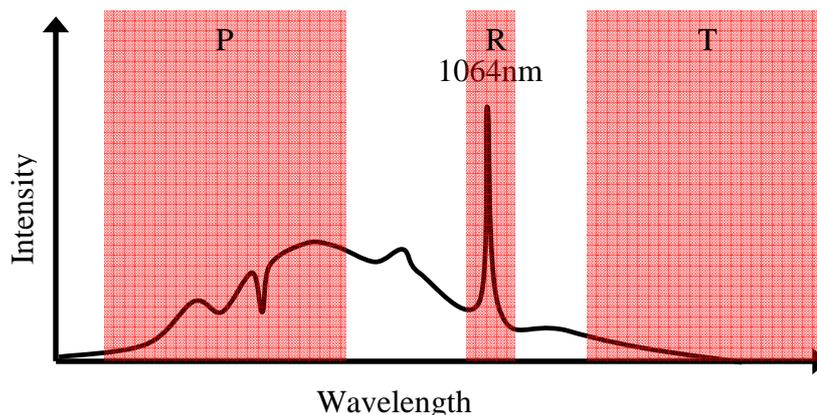
*Fig.2 Typical intensity distribution of the electromagnetic signal from Nd:YAG welding, and the wavelength range of the three sensors.*
