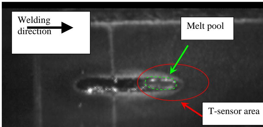
**Fig.8a** Image during OFF period in the centre of the weld
