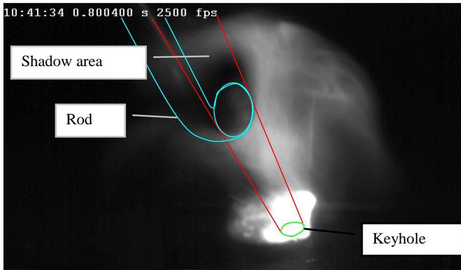
**Fig.14** Nonilluminated frame during welding.
