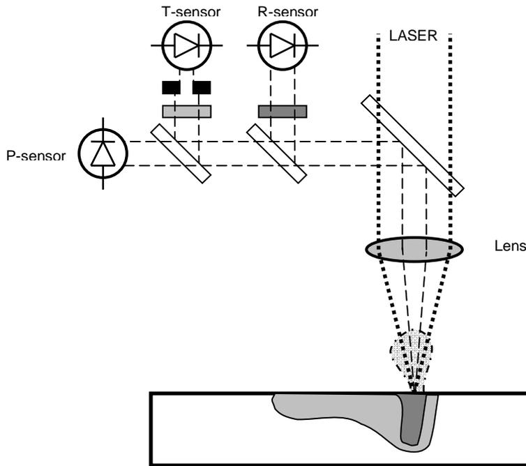
**Fig. 1** Standard concept of photodiode monitoring system.
