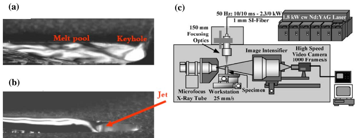
**Figure 5:** High speed imaging of the top side of the melt pool and keyhole [4]: (a) weld pool waves, (b) calmed weld through an additional gas jet directed to the keyhole rear side. (c) Example of a set-up for X-ray high speed imaging [7]
