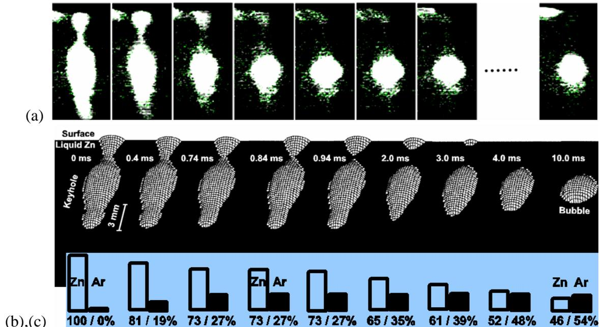
**Fig. 4:** Keyhole collapse towards a bubble after termination of a laser pulse: (a) time sequence of X-ray images of the keyhole (side view), (b) contraction predicted by the model, (c) calculated mixture of metal vapour (Zn) and shielding gas (Ar) in the keyhole/cavity [7]
