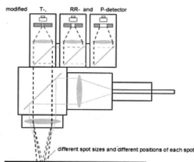
**Fig. 1.** Principle for photo-diode multi-sensor arrangement [6]
