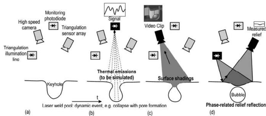
**Fig. 3.** Proposed method for identifying the surface geometry and motion (defect cause) as origin of resulting irradiation signal changes and in turn derivation of a theoretical context: (a) 3 observation instruments, (b) monitoring photodiode (emissions to be simulated by ray tracing), (c) high speed imaging (qualitative), (d) triangulation profile (quantitative)
