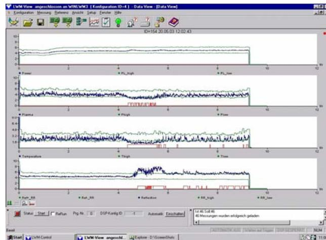
*Fig. 2. Sensor signals form a multi-sensor process monitoring system indicating weld defects, due to a large gap in a lap welding application, as the actual signal is outside the reference signal levels*
